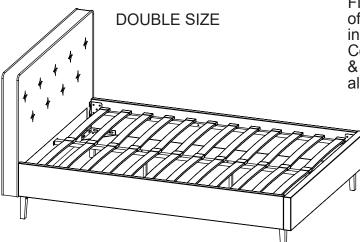
Fit single plastic caps (9) to each end of a pair of slats (8) then slide into the double cap (10) in the centre.
