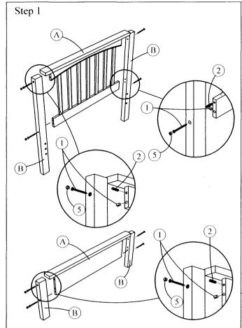
Assemble the bed frame headboard and footboard component as shown and tighten all bolt.
