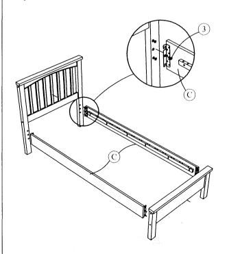
Attach the side rail (C) to the headboard and footboard using bolt (3) and allen key (G) as shown ensuring the pre-drilled holes on the side rail are facing up.
