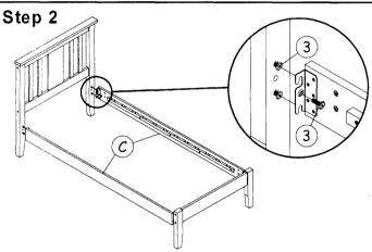
Fix bolt '3' (upper & lower bolts) into position on wood post as shown. After that, hook the side rail to the bolt and fix center bolts '3' as shown.
