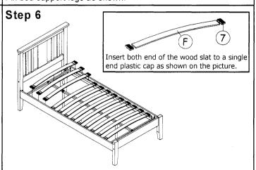
Once wood slats have been inserted into the plastic caps, fix one end of wood slat into the hole of side rail by pressing it accordingly to the defaults holes and the other end to the other side rail holes. Ensure the plastic cap's pin aimed to the hole.
