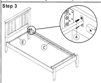
Fix cross bar 'E' to the side rail with bolts '4' as shown.
