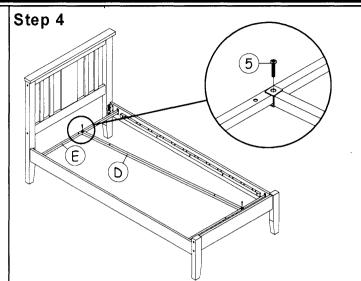
Fix center bar 'D' to the cross bar 'E' with bolt '5' as shown.
