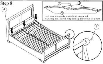
Once both wood slats have been inserted with the plastic caps, fix it on the wood side rails and center bar by pressing it accordingly to the default holes. Ensure the plastic cap's pin is aimed to the hole. At last fix wood button J.
