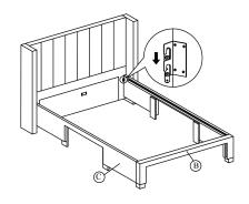
Attach side rail (C) to headboard (A) and footboard (B) by pushing the bracket down to fit it.
