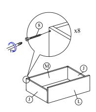
Tighten the side rail side panel (J) to the side rail front panel (L) and side rail back panel (M) with screws (8) using screw driver (not included).
