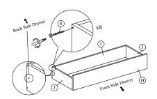
Tighten the footboard side panel (J) to the footboard front panel (H) and footboard back panel (I) with screws (8) using screw driver (not included).
