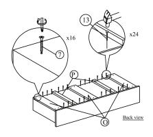
Tighten the bottom panel support (O & P) with screws (7) using screw driver (not included). Attach the bottom panel with Nail (13) using the hammer (not included).
