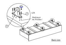
Tighten the roller (9) with screws (5) using screw driver (not included).
