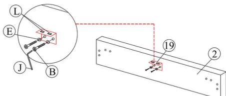
1. Position the Footboard (2) on a stable surface with the inner side facing up.
