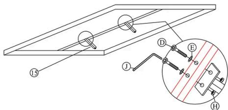
1. Align the Support Legs (15) with the holes at each end of the bar.
