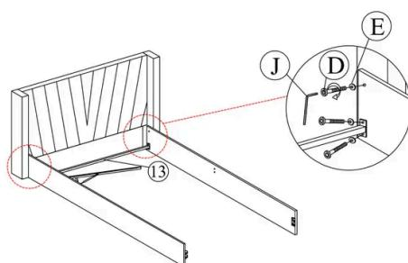
1. Bring the assembled Headboard (1) with wings into position.
