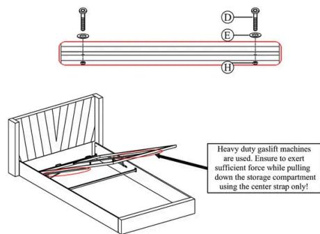
1. Carefully lift the metal slat frame (already connected to the gas lift machines).
