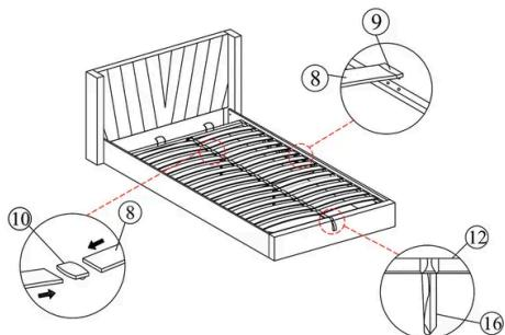
1. Insert the Wood Slats (8) into the Single Close Ended Clips (9) on both sides of the slat frame.
