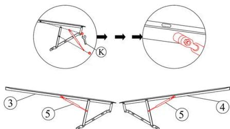
1. Position the Left Gas Lift Frame (3) and Right Gas Lift Frame (4) on a flat surface.
