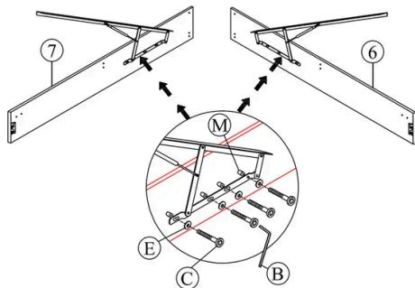
1. Align the Left Gas Lift Frame (3) with the Left Side Rail (7) and the Right Gas Lift Frame (4) with the Right Side Rail (6).
