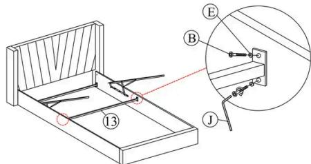
1. Locate the Side Rail Connector Metal Bars (13) and position them between the Left (7) and Right (6) Side Rails, near the footboard end.
