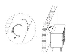
Secure the cabinet to the wall by attaching the tie for the anti-tilt bracket (D) to the bracket on the wall.
