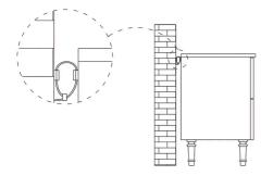
Ensure the tie for the anti-tilt bracket (D) is securely fastened to both the cabinet and the wall bracket. This will stabilize the cabinet and prevent it from tipping over.
