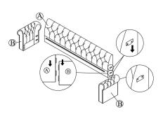
Attach the arm (B) to the back rest (A) by pushing the bracket down to fit it.
