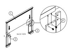
Fix head bottom leg left & right to the head board top with minifix 'F' as shown .
