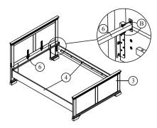
Fix cross bar '6' to the side rail with bolts 'B' as shown.
