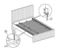
Affix the Slat (D) to the side rail support wood and the center rail (E) . Tighten all the  $4\ corner$  .
