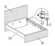
Attach side rail (C) to footboard (B) and headboard (A) by pushing the bracket
