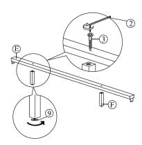
Attach the support legs (F) to the center rail (E) of the bed as shown.
