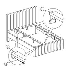
Slide the center rail (E) to the headboard (A) and footboard (B). Tighten screws (4) using screw driver (not included) to the headboard (A) and footboard (B).
