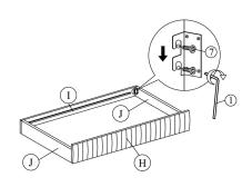
Attach trundle side panel (J) and trundle front panel (H) to trundle back panel (I) by pushing the bracket down to fit it.
